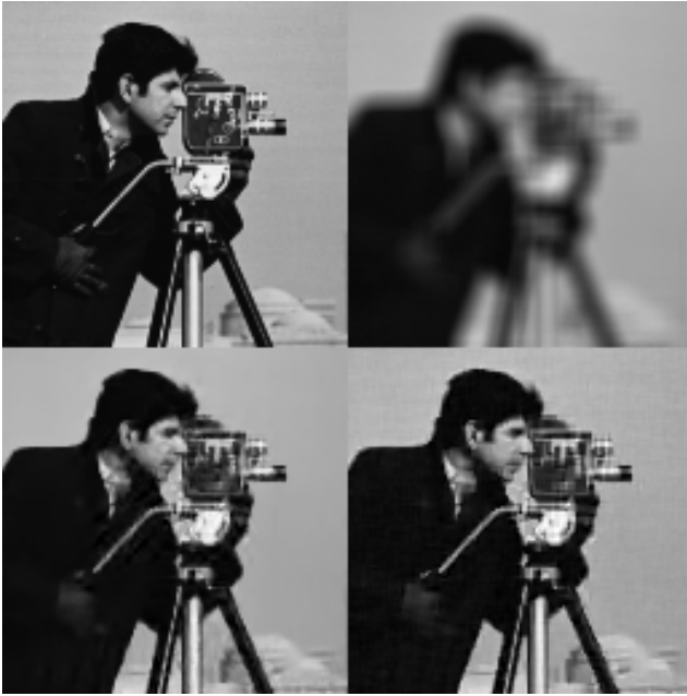
Fig. 2. From left to right and from top to bottom: (a) Crop from Cameraman ; (b) Simulated observation using a 9 \times 9 uniform kernel, with noise variance 0.308 (3rd. experiment); (c) Previous best result, from [9] (8.57 dB ISNR); (d) Our result (9.10 dB).
